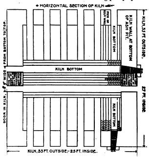
loose, will get burned after two kilns are burned, and then the inside being daubed with sandy clay grout, as it should be, the walls will be sufficiently open to prevent heating through; that being the object of the hollow in solid wall, so as to save heat.
